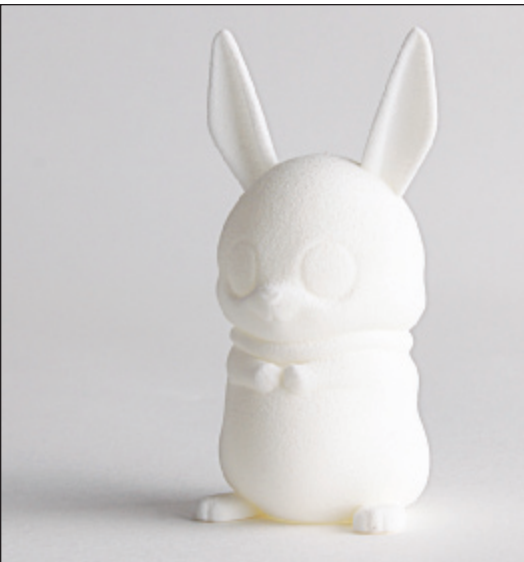
◀ Fused nylon powder, via selective laser sintering.
