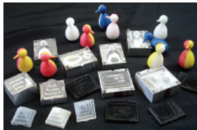
Stanavich is also using his PCNC 1100 to machine the permanent molds for toys he uses as unique calling cards for the shop.
