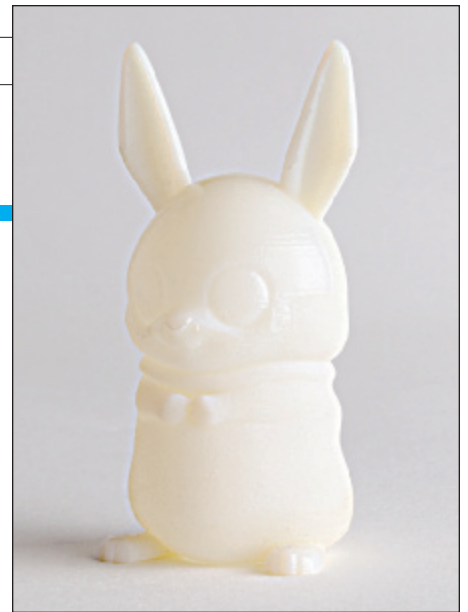
⚡ UV-curing acrylic, via photopolymer jetting.
